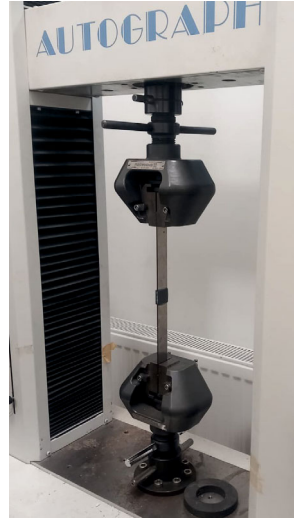
Fig. 3. Tensile test setup.
